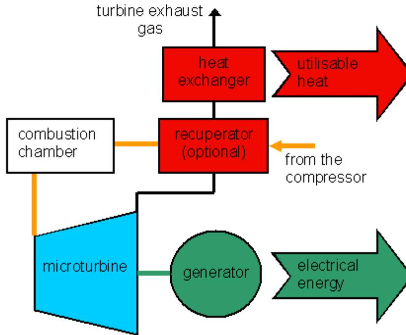
Besides block heat and power plants equipped with gas or diesel engines, recently also microturbines are gaining importance as another variant of a block CHP plant. If, however, high waste heat temperatures are required the microturbine represents the better solution.
