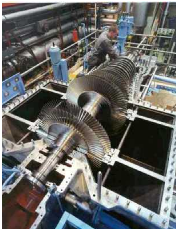
Figure 4: Rotor of a steam turbine with 8 MWel (Source: Peter Brotherhood Ltd)
