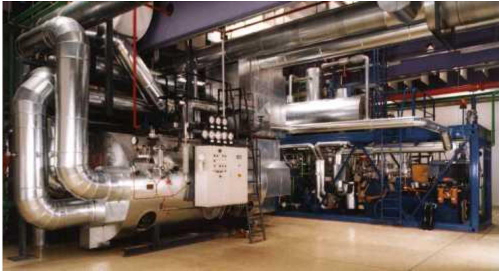
Figure 37: Prototype plant for a steam screw-type engine at the University of Dortmund (Source: UNI Dortmund)
